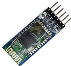
The HC-05 Bluetooth Module is a straightforward Bluetooth SPP (Serial Port Protocol) module created for the establishment of transparent wireless serial connections. Because it communicates serially, interacting with a controller or a PC is simple. With the ability to switch between master and slave modes, the HC-05 Bluetooth module can neither receive nor send data.
