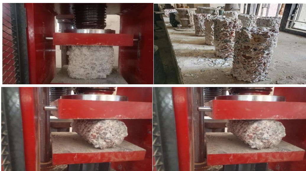
Fig 5.4: Concrete cube and cylinder compressive strength test and split tensile strength test after acid curing
