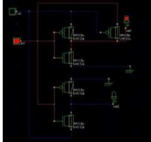
Apply Input A=1 and B=1 and verify the output. The expected output should be S=0 and C=1
