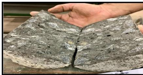
Fig. 4.7- Split tensile failure of SCC-100/0 mix
