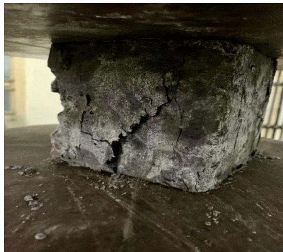
Fig. 4.5- Compressive failure of SCC-100/0 mix
