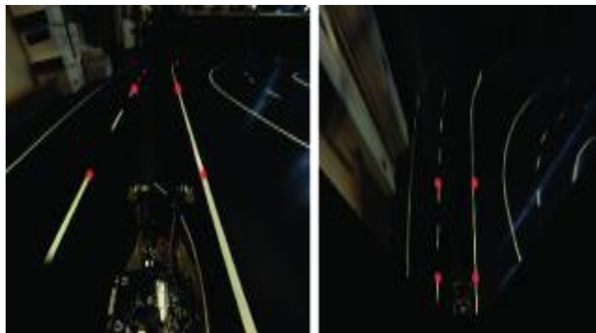
Fig.5: Bird's eye view transformation process using four mapping points illustrated in red.
