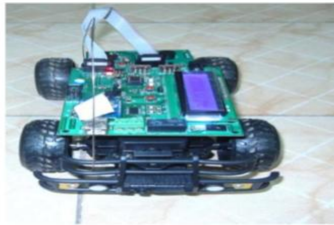
Fig. 2. The proposed mobile sink – a classical vehicular robot design.
