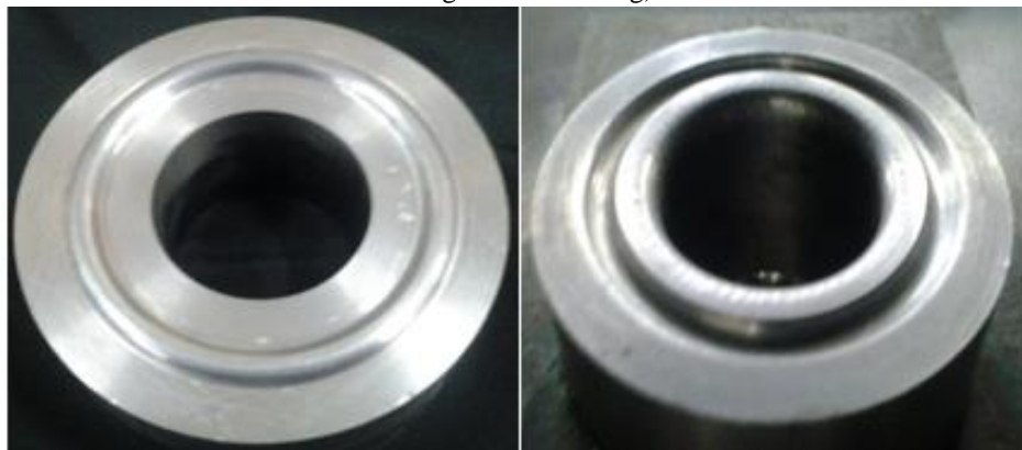
Fig 1.4 Upper die and lower die for stretch forming
