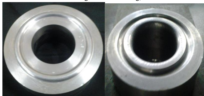
Fig 2.6 Upper die and lower die for stretch forming
