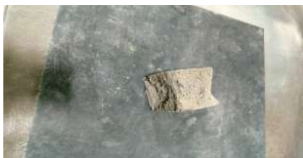
Figure 4: Broken cube after experimentation.
