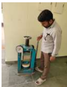
Figure 3: Breaking of cube sample during compression test.
