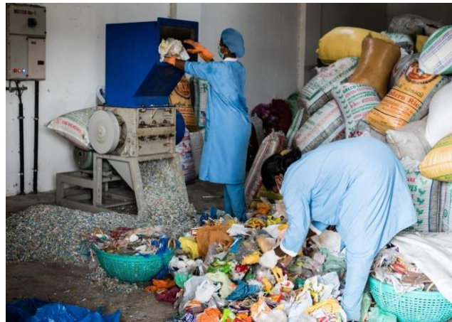
Figure No 6. Shredding & Cleaning process
