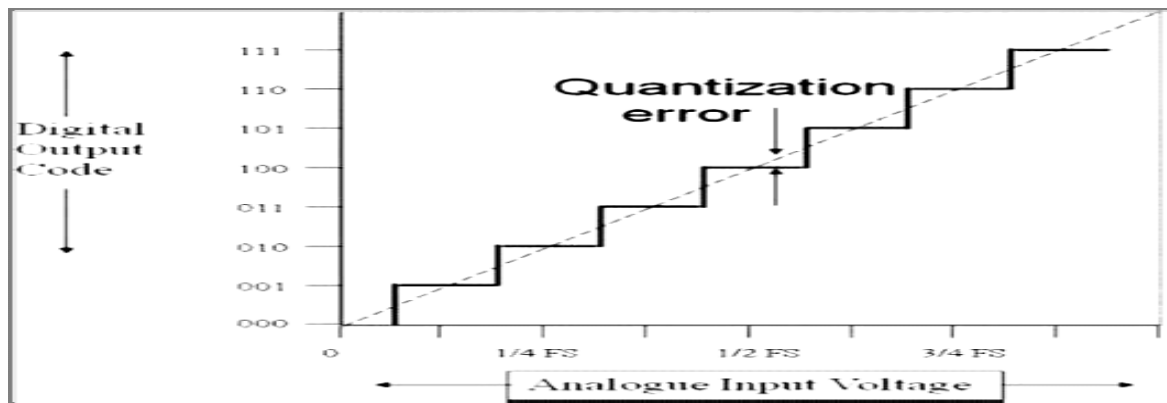
Fig.2 Variation of Quantisation error as a function of signal voltage
