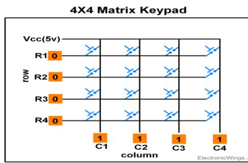
4x4 Keypad PinoutThe columns and rows make up the matrix layout of the keyboards. The columns and rows make intimate contact if a key is pushed. If not, then rows and columns don't have any significance.
