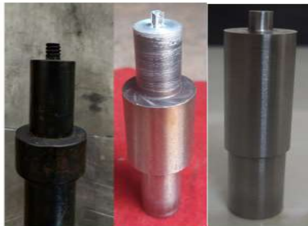
Figure 2 Threaded Cylindrical, Square, and Clindrical tool pin profiles
