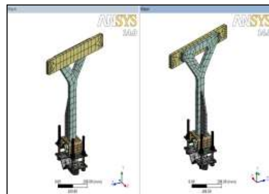
Figure:-Modified Design Of Blade CAD Model (meshing)
