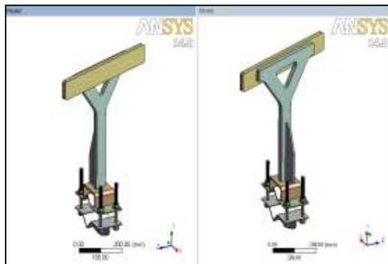
Figure:-Modified Design Of Blade CAD Model (Geometry)
