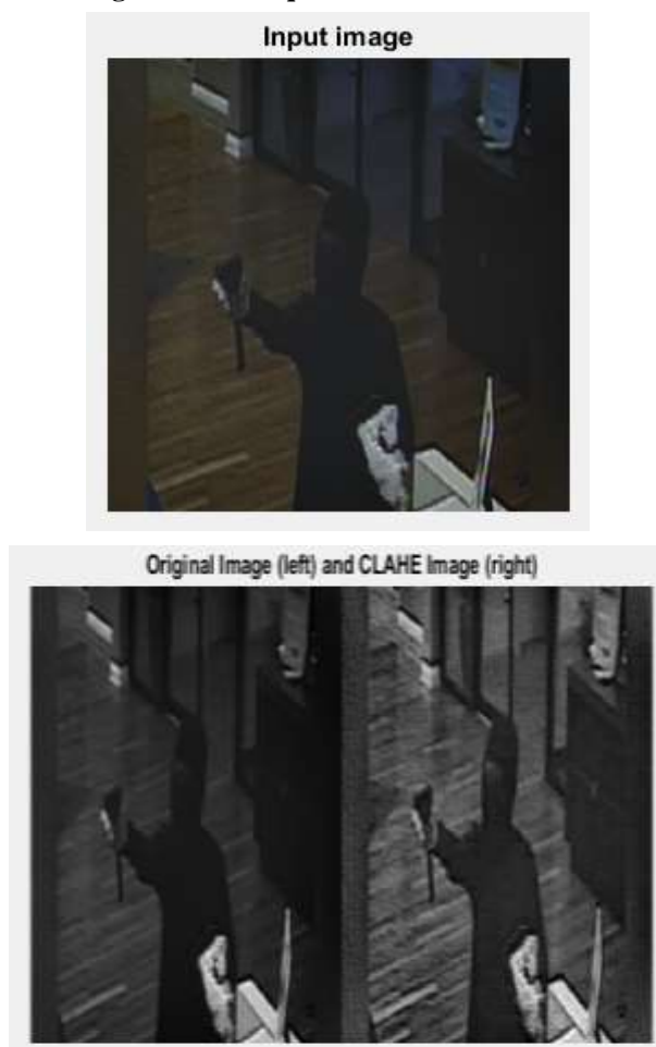
Figure 4.1: (a) Input selected image, (b) Original image in gray scale (left) and CLAHE image (right)
