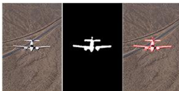
Figure 3. Detection and Outlining of an Aircraft using Segmentation and Morphology
