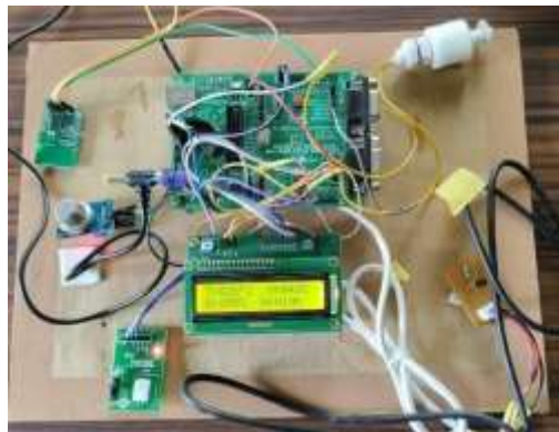
Fig.15. Transmitting Part-Sensors and LORA transmitted interfaced with the micro controller
