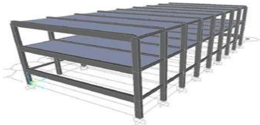
Fig 4.1 Model of function hall in SAP 2000
