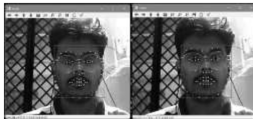
Figure 5. (a) Eyes are completely open with EAR value 0.35 and (b) Eyes are fully closed with EAR value 0.24
