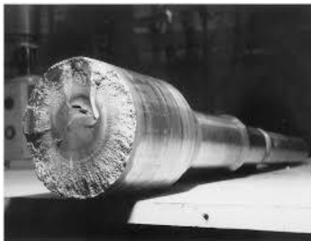
Fig. 2.4 (a) and (b) Broken part of pull rod and clevis
