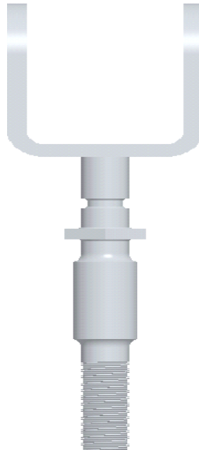
Fig.4.3 Existing pull rod
