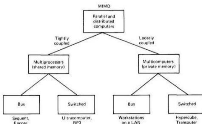
Although all distributed systems contain multiple processors, there are many alternative ways to combine them, and as Flynn (1972) knew 2 basic characteristics of to classify portable multiprocessor systems: the number of instruction streams and therefore the amplitude of the knowledge flow.
