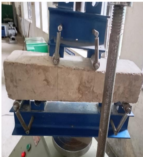
Fig 13: Flexural Strength Test of Beam
