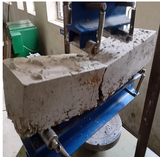
Fig 13: Flexural Strength Test of Beam
