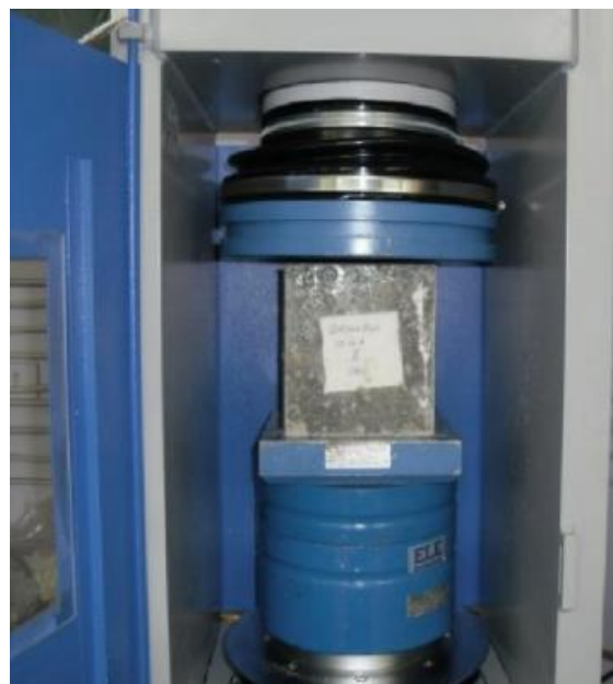
Figure 2: Representation of concrete compressive strength test
