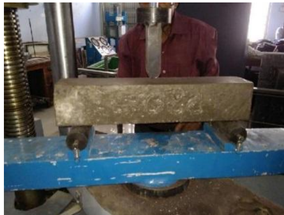
FIGURE. 3.2 Flexural strength test
