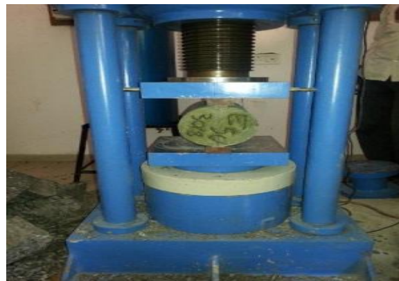
FIGURE 3.1 Test for Splitting Tensile strength
