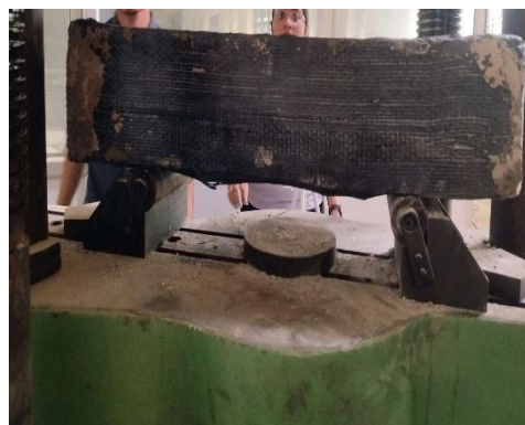
Fig 20. Debonding Failure on Fully Wrapped in 2 layers CFRP Beam
