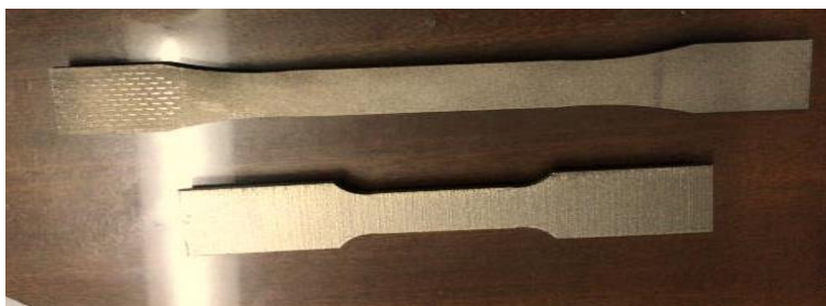
Figure 3. 2: Tensile Inconel specimens
