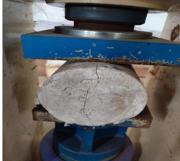
Fig.2 Split tensile strength
