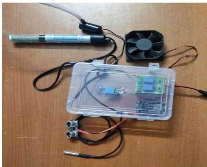
Fig.3.1. The hardware setup of the IoT-based water bodies monitoring system is shown.
