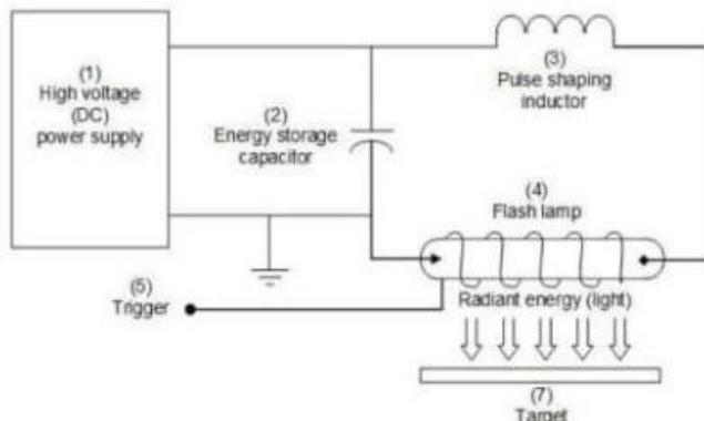
Functional diagram of a high – intensity pulsed – light system (Adapted from Xenon Corp., 2005)
