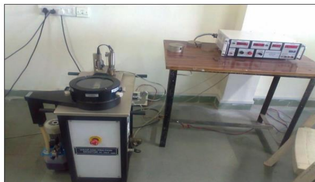
Fig. 4.1 Photograph of experimental set up (Tribometer TR-20LE).
