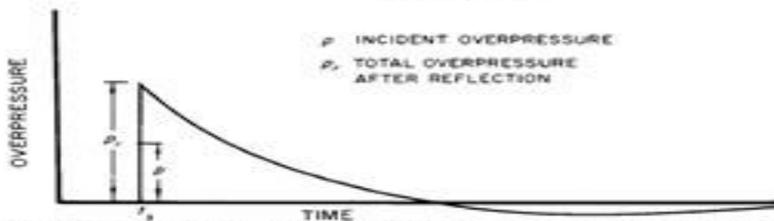
Figure 3.22. Variation of overpressure with time at a point on the surface in the region of regular reflection.
