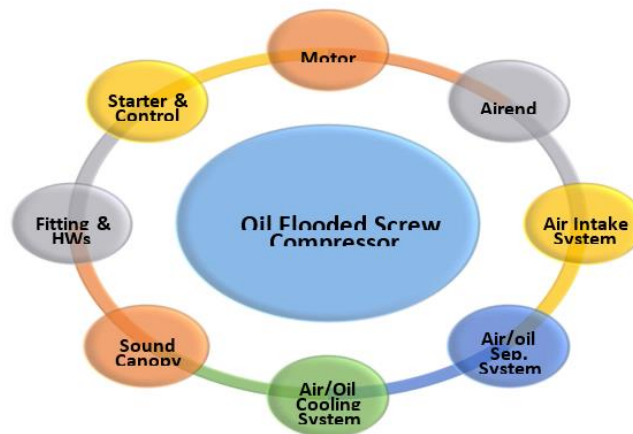
Fig.2. Schematic depiction of the components of an oil-flooded rotary screw compressor
