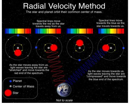
Diagram detailing the Radial Velocity (aka. Doppler Shift) method. Image © Las Cumbres Observatory
