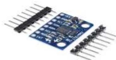
MPU6050 is a micro-electromechanical system (MEMS) sensor that combines a 3-axis gyroscope and a 3-axis accelerometer in a single chip. The MPU6050 is commonly used in a wide range of applications, including robotics, drones, gaming controllers, and motion sensing devices.
