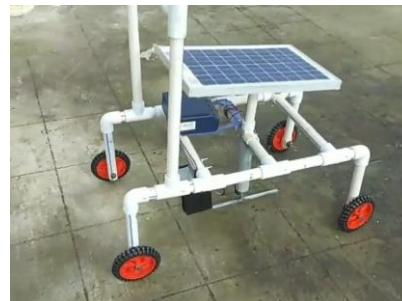
External Frame Work: The external frame work is having 1 inch PVC hallow pipes, elbows and tees. The wheels are attached to the body as shown in fig. the blade is coupled to the shaft of the motor. The motor is attached to the body through the 1 inch by 1.5 inch PVC reduceroverall height of the model is 4.5 ft.
