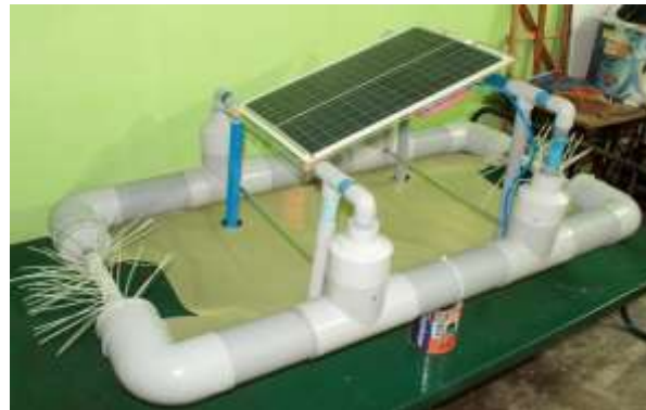
Fig .1 PVC Frame, Propeller Stem, Solar Panel, Electronics Storage, Solenoid valve,Axial Impeller
