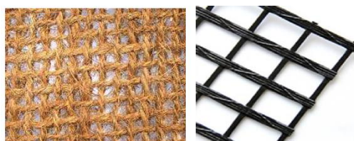
Figure 3: Geosynthetics used (a) Woven Geotextile (b) Geogrid
