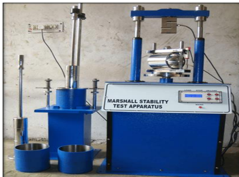
Figure 3.1 Marshall Stability Test Apparatus.
