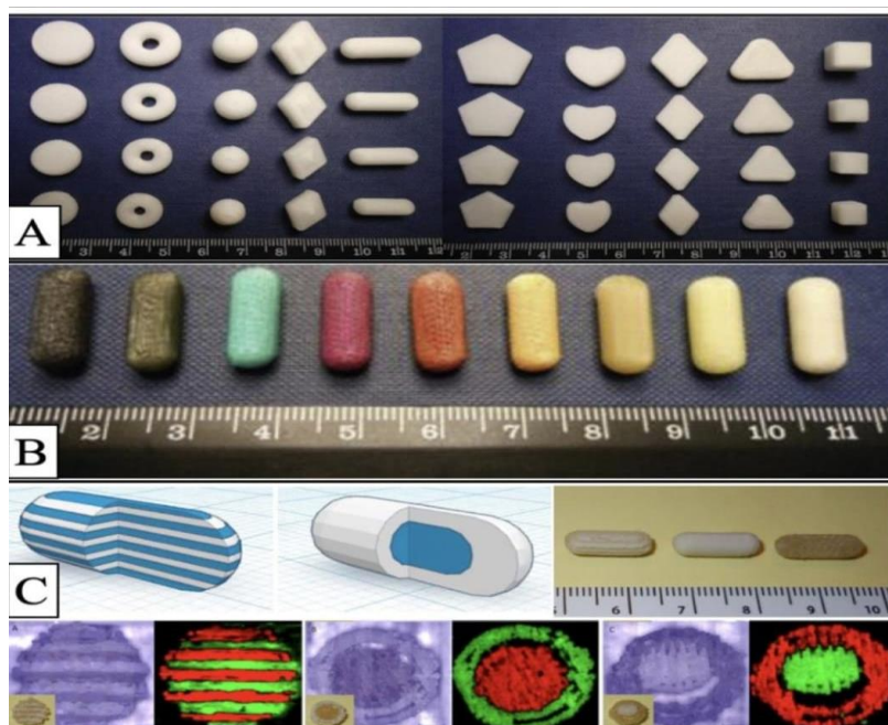
Figure 3. Images of various types of tablets prepared by FDM technology: (A) Images of 3D-printed tablets with different shapes and sizes [42]; (B) images of 3D-printed tablets in capsule form with different colors [42]; (C) sectioned multilayer device and sectioned DuoCaplet (caplet in caplet) model images, 3D-printed preparations, and white light and 2-dimensional Raman mapping images [85]. Figures were reproduced and modified with permission from [43].
