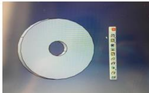
Figure 2: Circular grain cross section using Auto CAD
