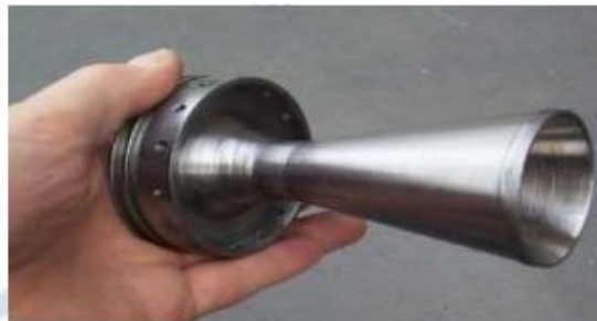
Figure 5: Mild steel nozzle
