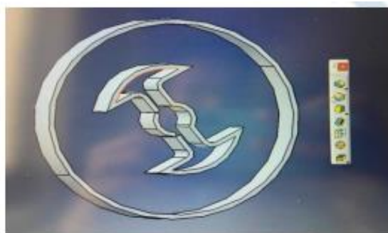
Figure 3: Double anchor grain cross section using Auto CAD
