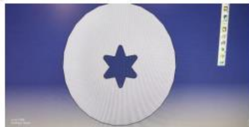
Figure 1: Star grain cross section using Auto CAD
