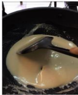
Figure. 6 Rocket Candy heating in the PVC propellant electric pot.
