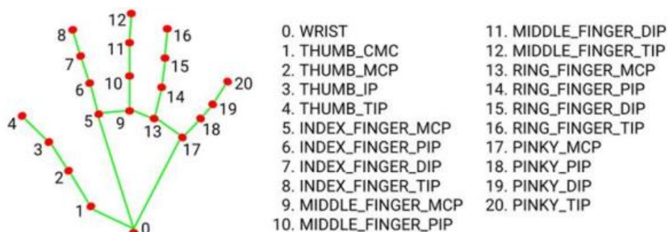
Fig. 1 The points predefined for the hand to recognize the hand gesture.
