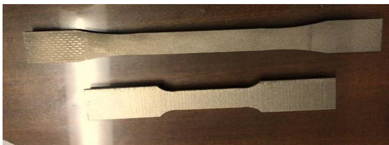
Figure 3. 2: Tensile Inconel specimens
