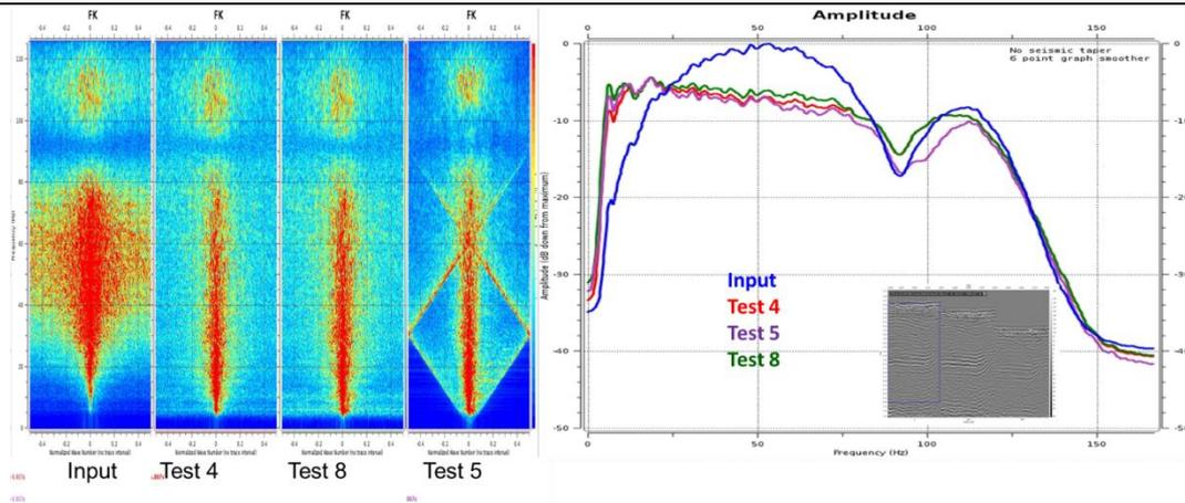
**Figure 10:** Near channel gather FK spectra show aliasing with RC increment in Test 5. This aliasing effect is not observed in Test 8 (variation of the RC)
