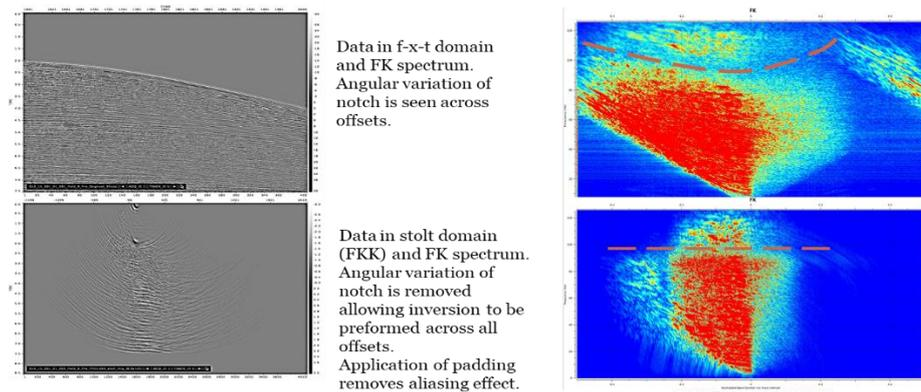
**Figure 4** Data in f-x-t domain (above) and FKK domain (below). Deghosting is done in the FKK domain where the near to far offset is better aligned for improve deconvolution of ghost energy
