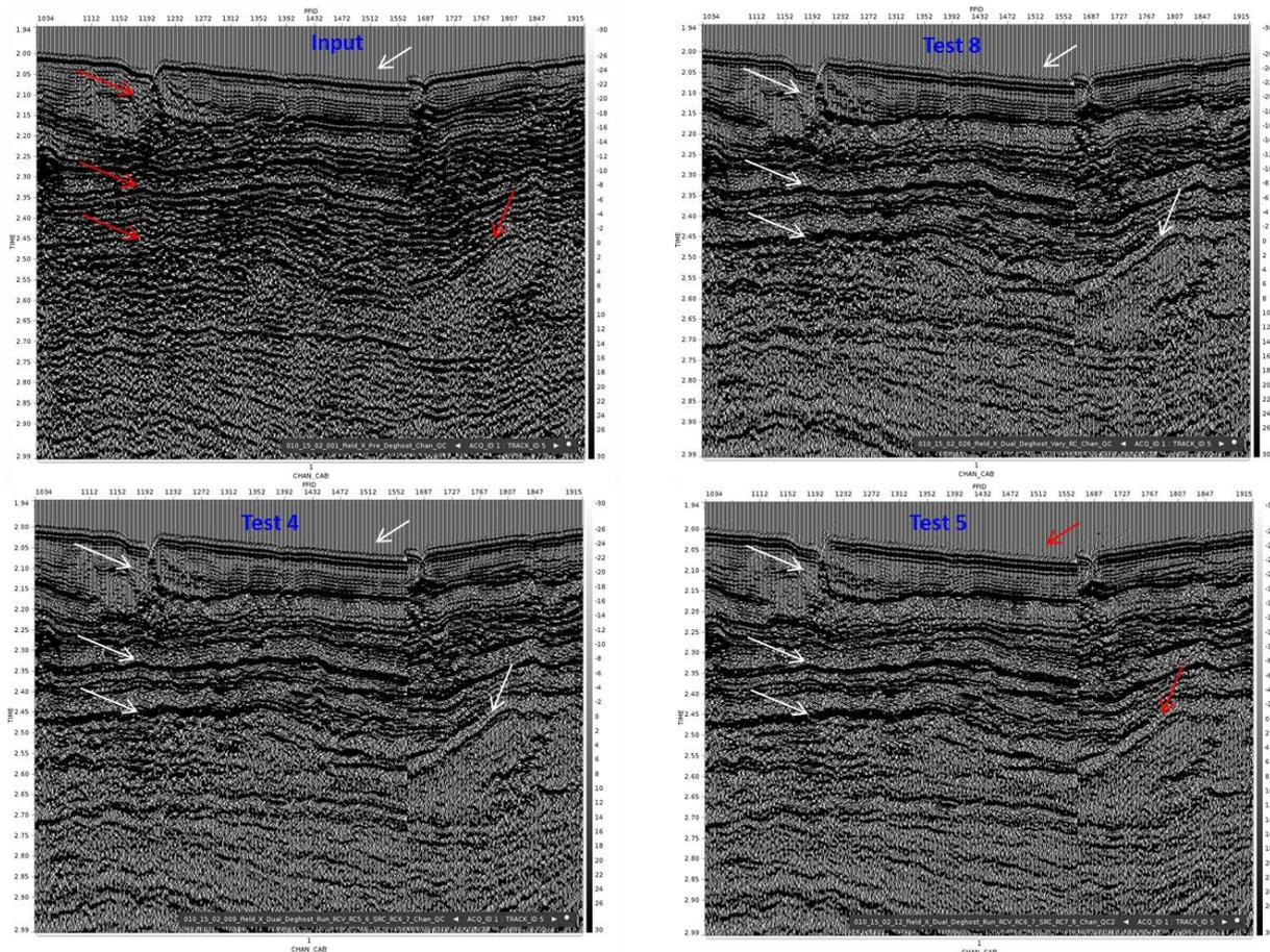
**Figure 9:** Near Channel gathers displays appears to show correction of phase distortion of higher frequencies observed in Test 5 near the water bottom with the use of Test 8 deghosting
