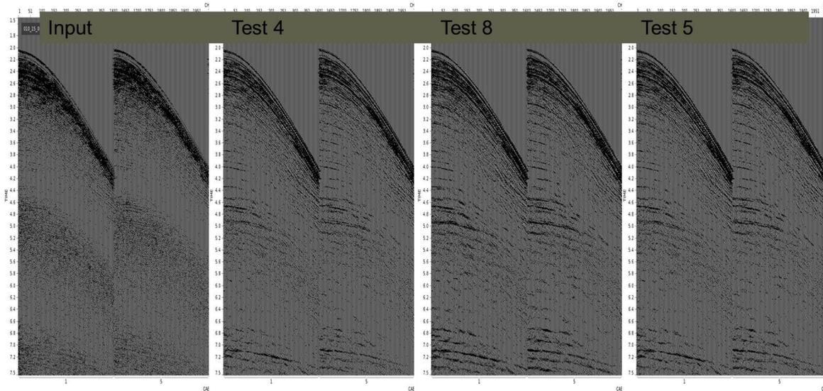
**Figure 8:** Shot gathers of data before and after deghosting. Signal appears more enhance with use of Test 8 varying RC across the frequency range
