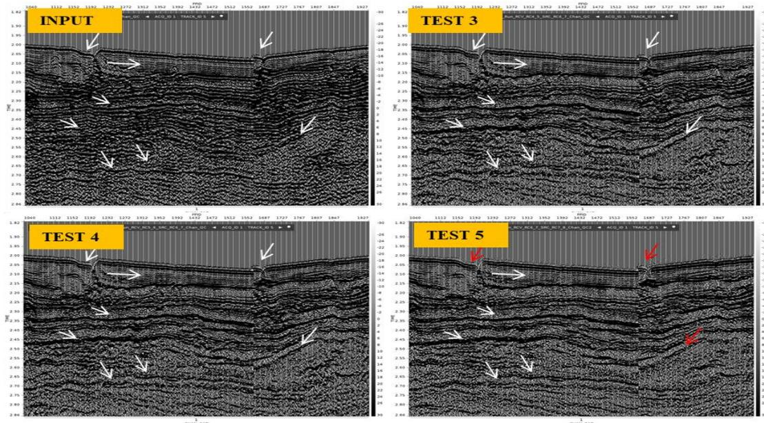
**Figure 7:** Near Channel Gatherers of Tests 3 – 5. Low frequency seen to improve with higher RC estimation but higher frequencies signals appear less optimal (red arrows) with increasing RC estimation
