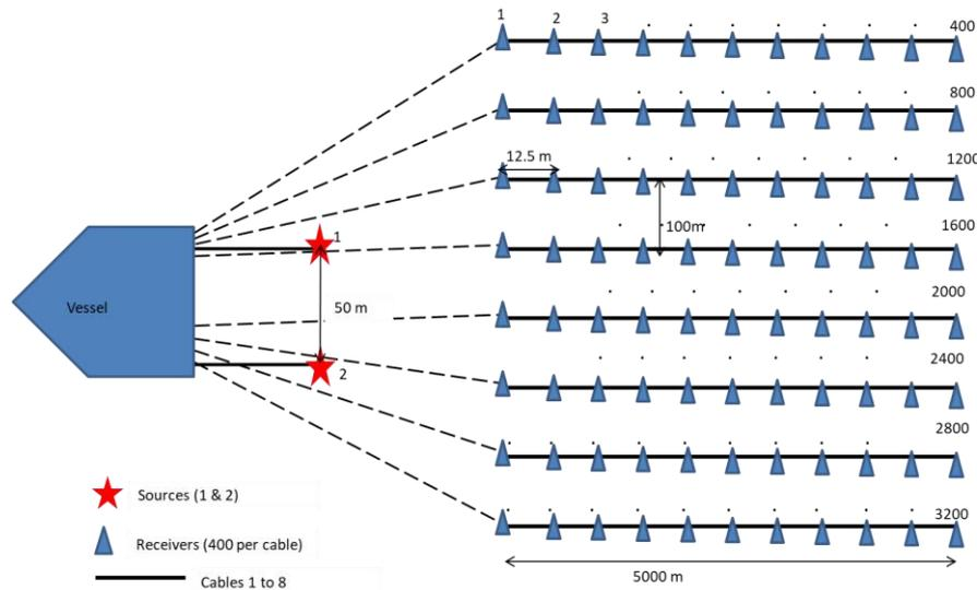
**Figure 2** Cartoon representation of acquisition spread of research data based on SEG Y header information
