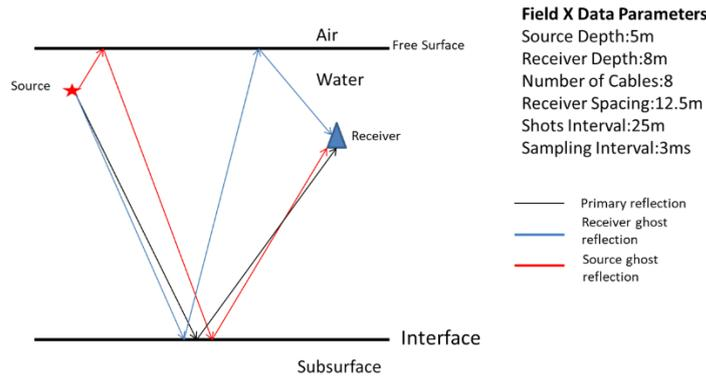
**Figure 1** Cartoon illustration of receiver and source ghosts generation
