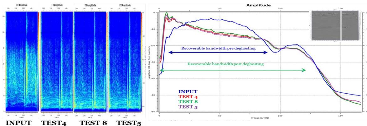
**Figure 12:** Pre-migration 3D stacks spectra FX and amplitude spectra without Q compensation show broadband enhancement of the data with deghosting
