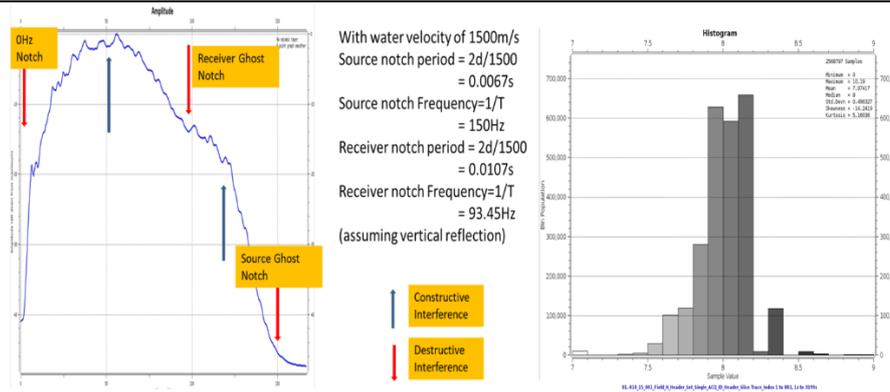
**Figure 3** Amplitude spectrum of input data with constructive peaks and destructive notches caused by source and receiver side ghosts interferences (Left). Right is histogram of receiver depths.
