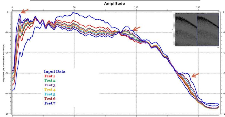
**Figure 5:** Amplitude spectra of shot gathers from Tests 1 -7. Spectrum at lower frequency appears boosted with increasing RC while the amplitude spectrum appears more distorted with increasing RC estimation (arrow indication Test 7 spectrum).
