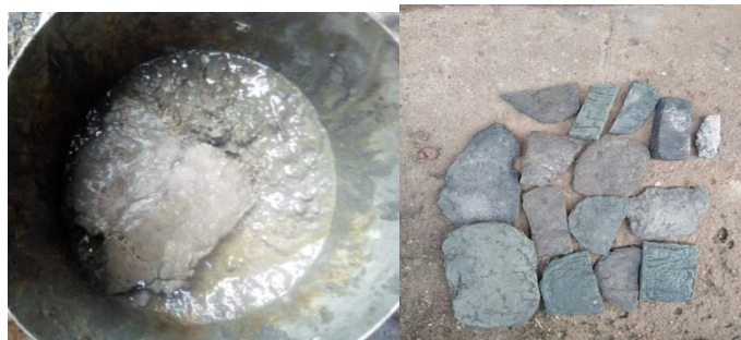
Plate 3: Molding of PP/PBA/HSS Composites Plate 4: PP/PBA/HSS Composites
