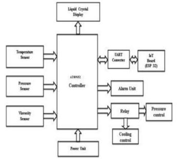
A system for monitoring and controlling industrial processes. It uses sensors to track temperature, pressure, and viscosity, with a microcontroller managing the data. An IoT board enables remote access, while a display and alarm unit provide real-time feedback and alerts. Actuators, like relays, adjust pressure and cooling as necessary for optimal operation. Overall, this setup enhances efficiency and safety in industrial settings.
