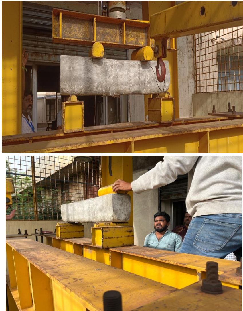
Figure 11: Testing of load framing using double point load.
