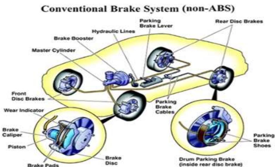
**Figure 1:** Disc brake system location in a car.
