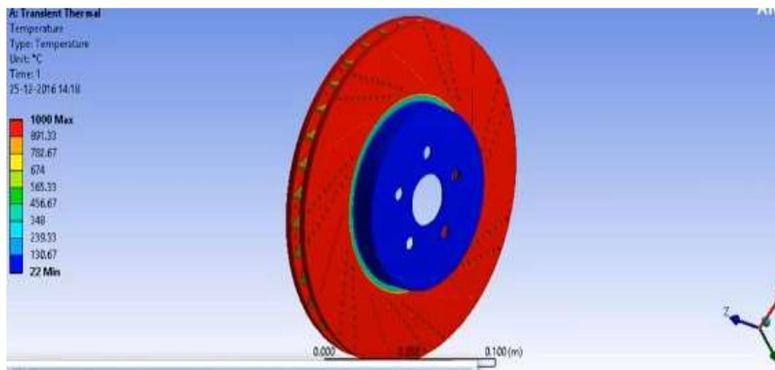
Fig 7 Maximum Temperature distribution
