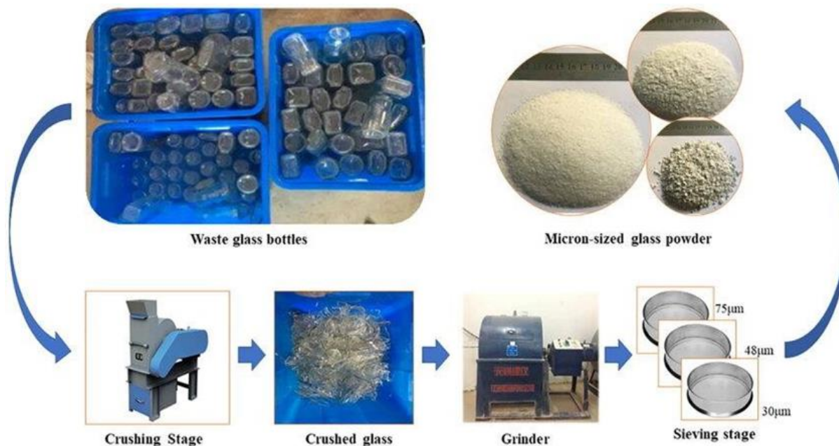
Figure 7 Process involved in converting glass to glass powder
